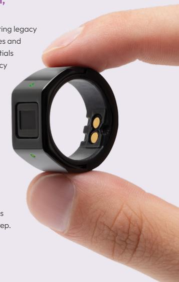
Token Ring secures user credentials by safely storing them directly on the ring. With a 508-dpi capacitive touch fingerprint sensor for on-device biometric matching, Token Ring delivers the highest level of security available.
