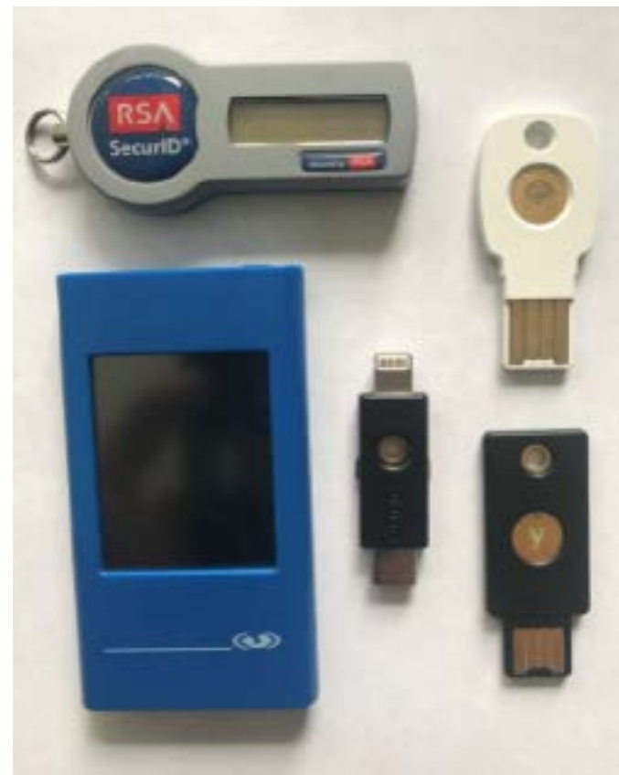
Various hardware keys used for MFA, including the latest Fido-support keys along the right side and RSA's latest SecurID. (credit: D.Strom)
